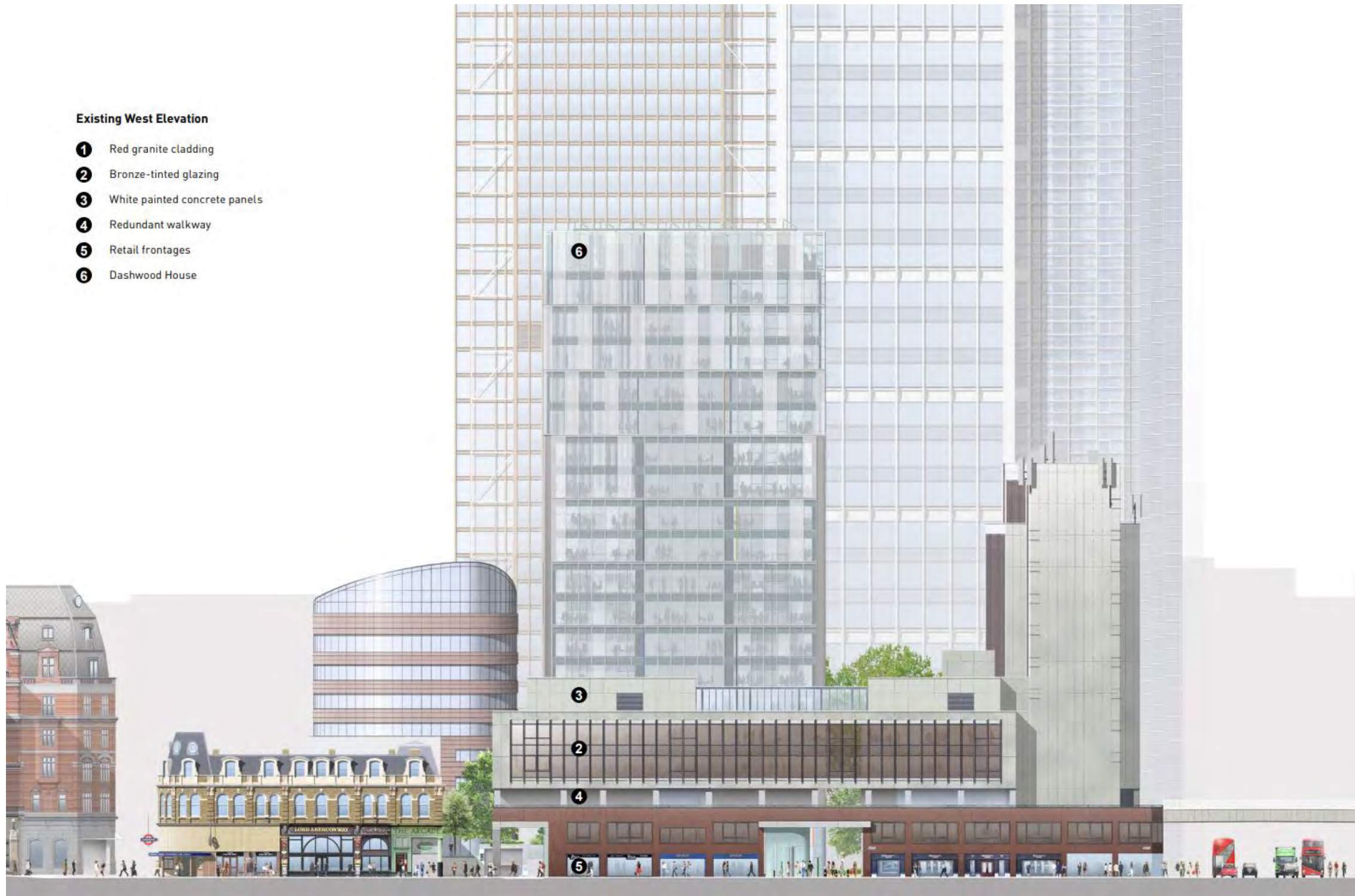
Existing West Elevation – Old Broad Street
